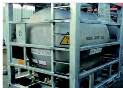
Helifuel Offshore Tank
